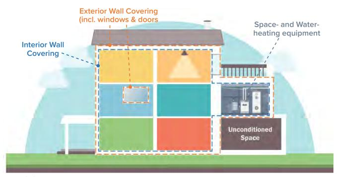
The **building thermal envelope** is the parts of a building (e.g., exterior walls, floors, ceilings, roofs) that enclose conditioned space or provide a boundary between conditioned and unconditioned space. **Conditioned space** is an area or room that is normally heated or cooled by equipment, whereas **unconditioned space** is any enclosed space within a building with no equipment to regulate temperature, like garages or attics.
